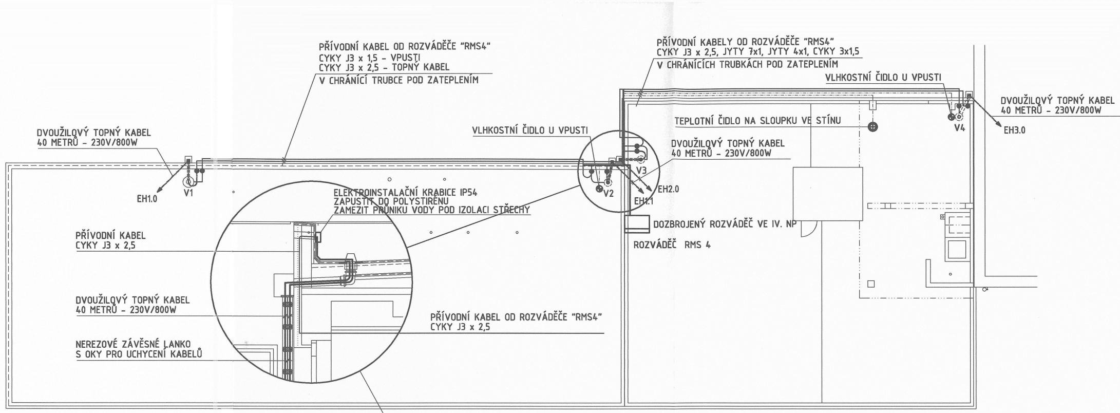
DETAIL PROSTUPU KABELU FASÁDOU DO VPUSTI A DEŠŤOVÉHO SVODU
