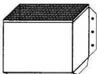
LISOVANÝ ROŠT S OCHRANOU HRAN PRO ZATÍŽENÍ 7,2 kN – 2 KS
